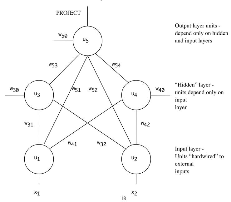
This is an example of a <u>feed-forward</u> layered network. By feed-forward, we mean that information flows one way, from the input toward the output.
